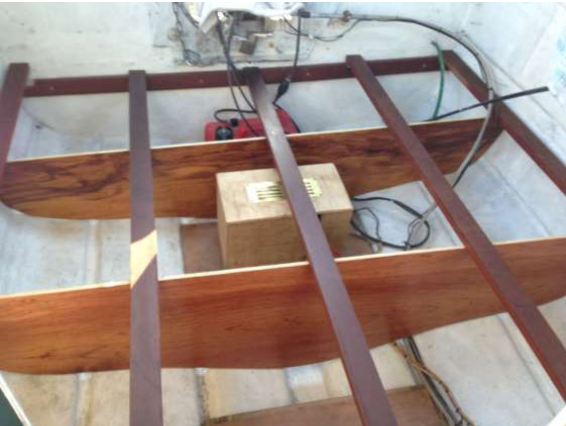
Need to trim the stringers height down slightly before final fix. 30/11/2017
