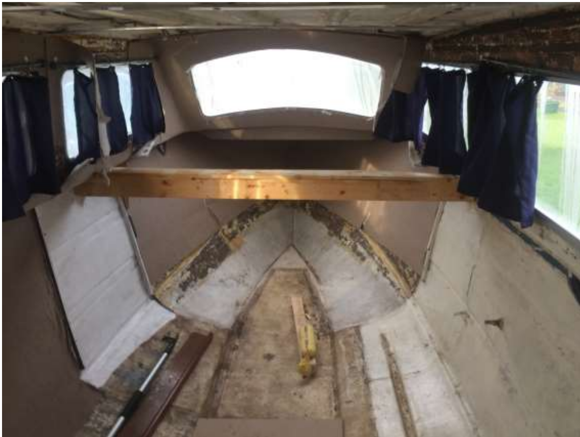
Just when we decided not to remove boat from the water. We detected a leak. A total strip out of the inside strengthening bar fitted ready for lifting out.
