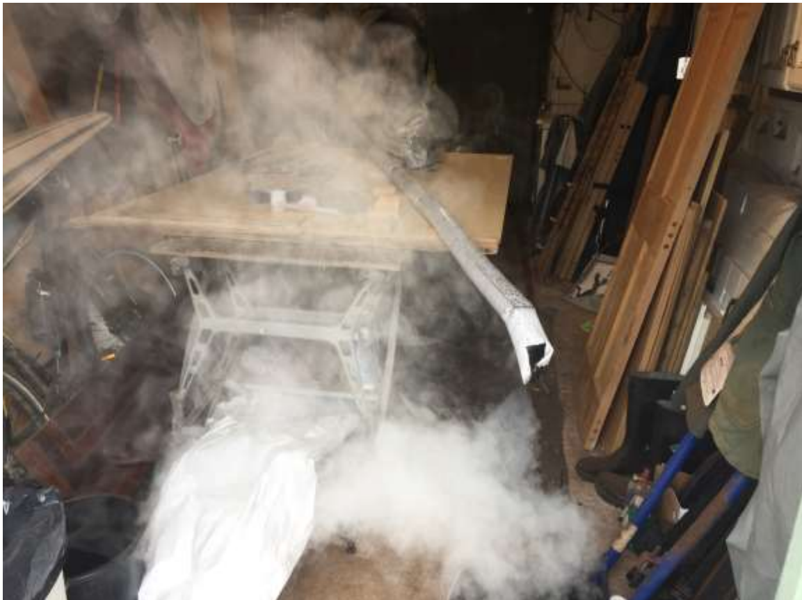
Mahogany batten placed inside layflat poly tubing and fed with steam from wallpaper stripper. Restricted steam flow out to ensure tubing inflated. Steamed for just over 1 hour.
