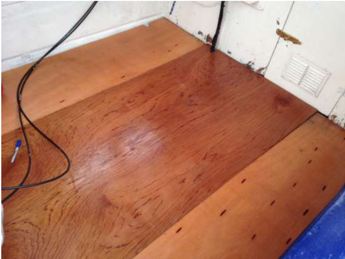
New stringers and floor supports installed in Skylark 03/12/2017. New plywood Floor installed temporarily for boat use over Xmas. 19/12/2017
