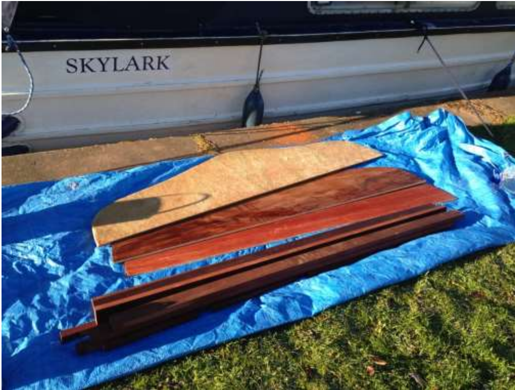
Floor stringers and supports on the canal bank. Below cabin stringer/wall fitted and bonded in forming a water tight bulkhead. 30/11/2017
