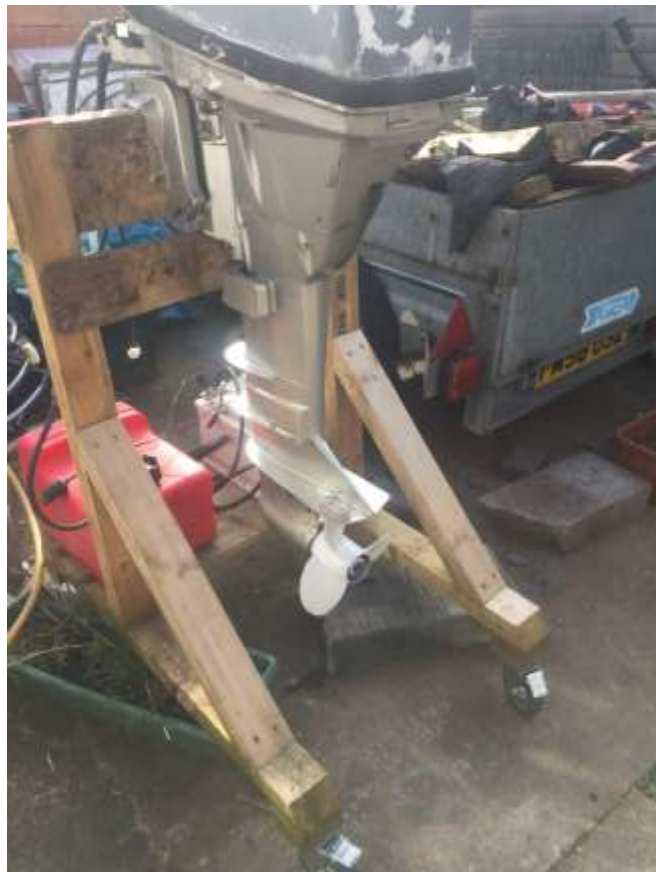
Gear box oil changed. Note the corrosion! (April 5 th 2020) Corrosion treated and primed and finished with Honda silver paint
