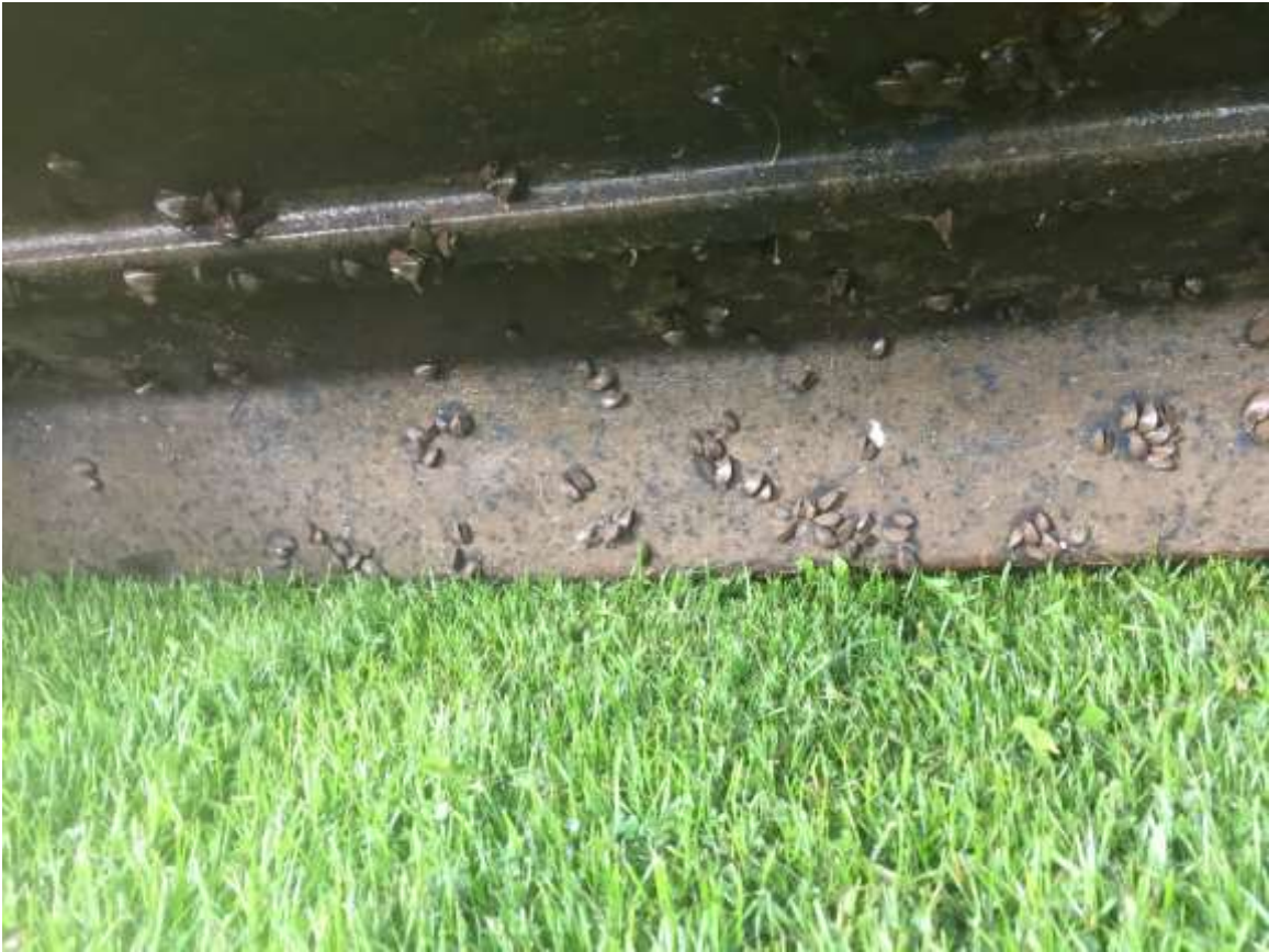
Had to scrape off all the shell fish (November 2019) Jet washed the hull prior to sanding
