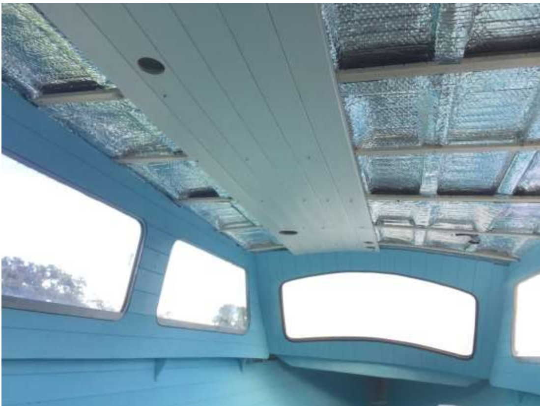
Another 20 boards being painted in the garage (23/09/20) Cladding the ceiling prior to re-wire (24/09/20)
