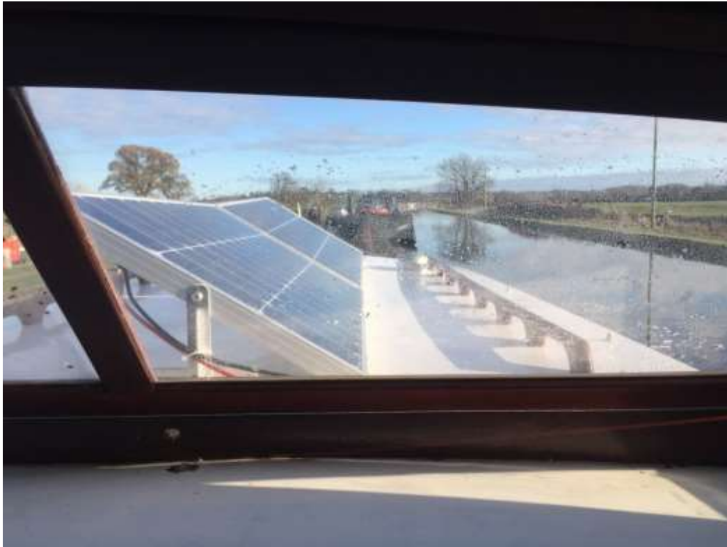
Two 100W solar panels fitted (27/11/20) Supplying new 105 AH leisure battery
