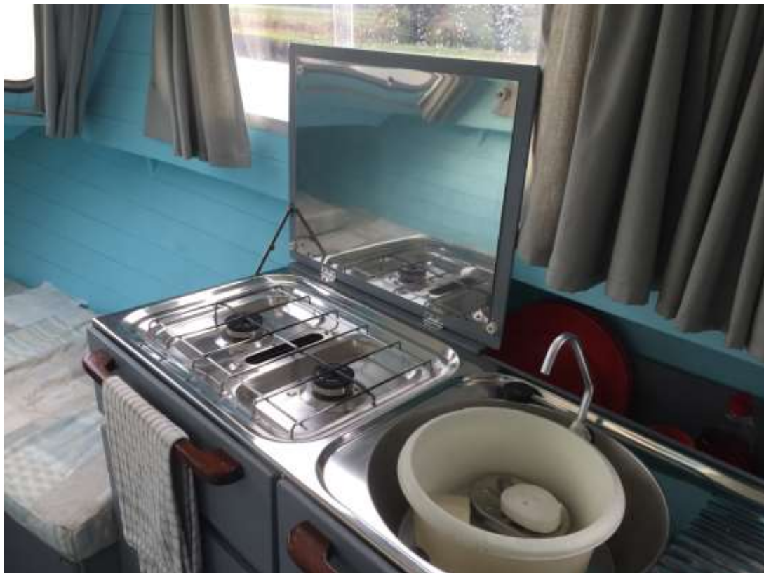
T&G under the bow deck. (15/11/20) Folding top fitted to cooker (28/11/20)
