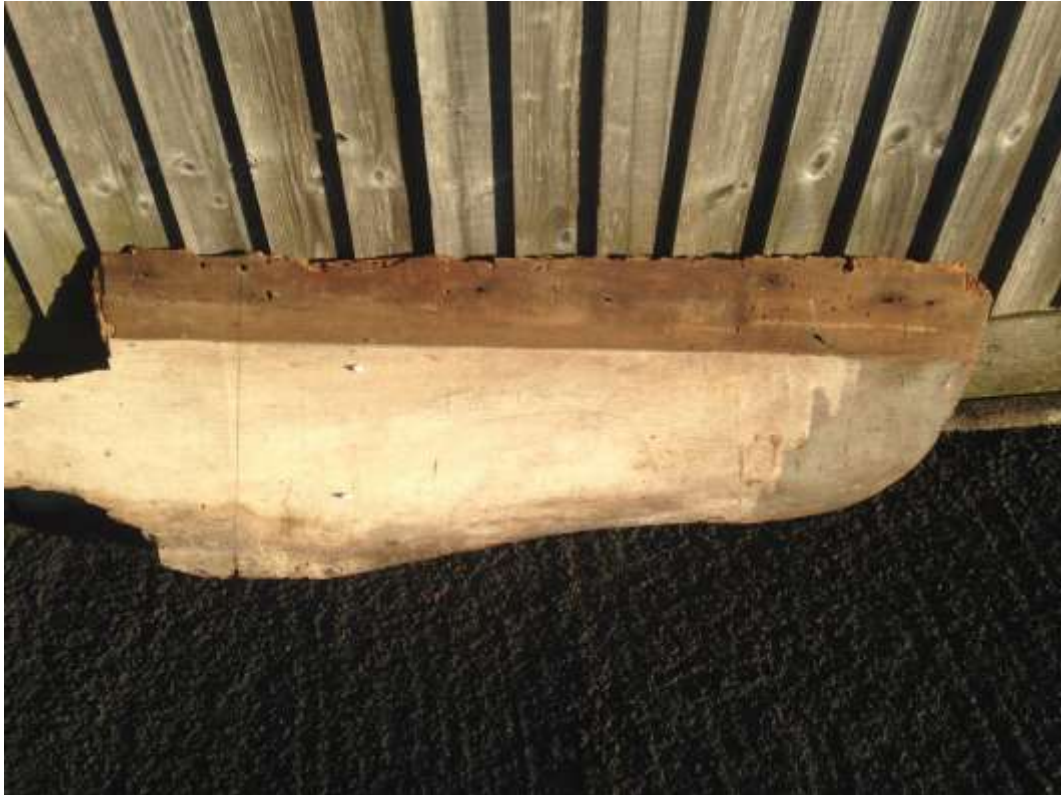
Most of the removed deck and framework. And below all I could salvage to form a half template. 27/10/2017
