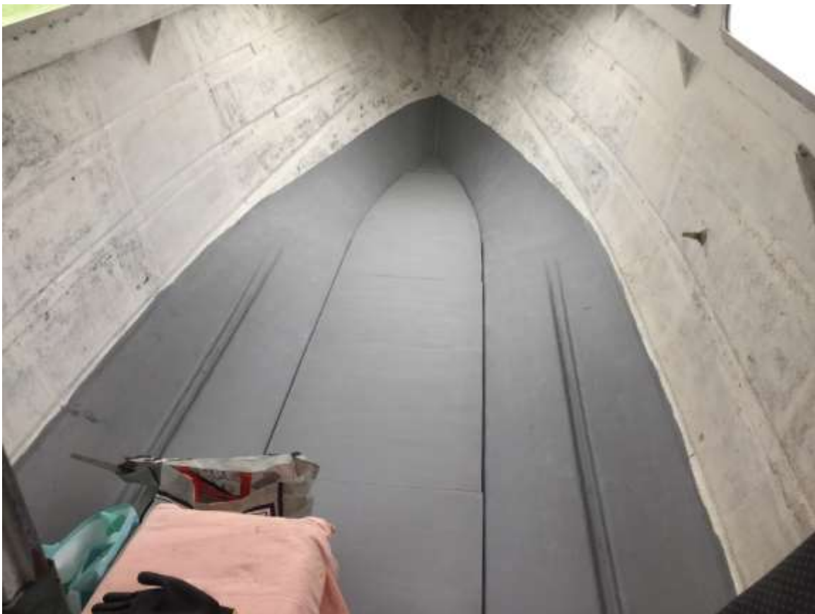
18mm plywood floor primed underneath & bonded to fibreglass (2/7/2020) Whole floor area painted with grey primer (2/7/2020)
