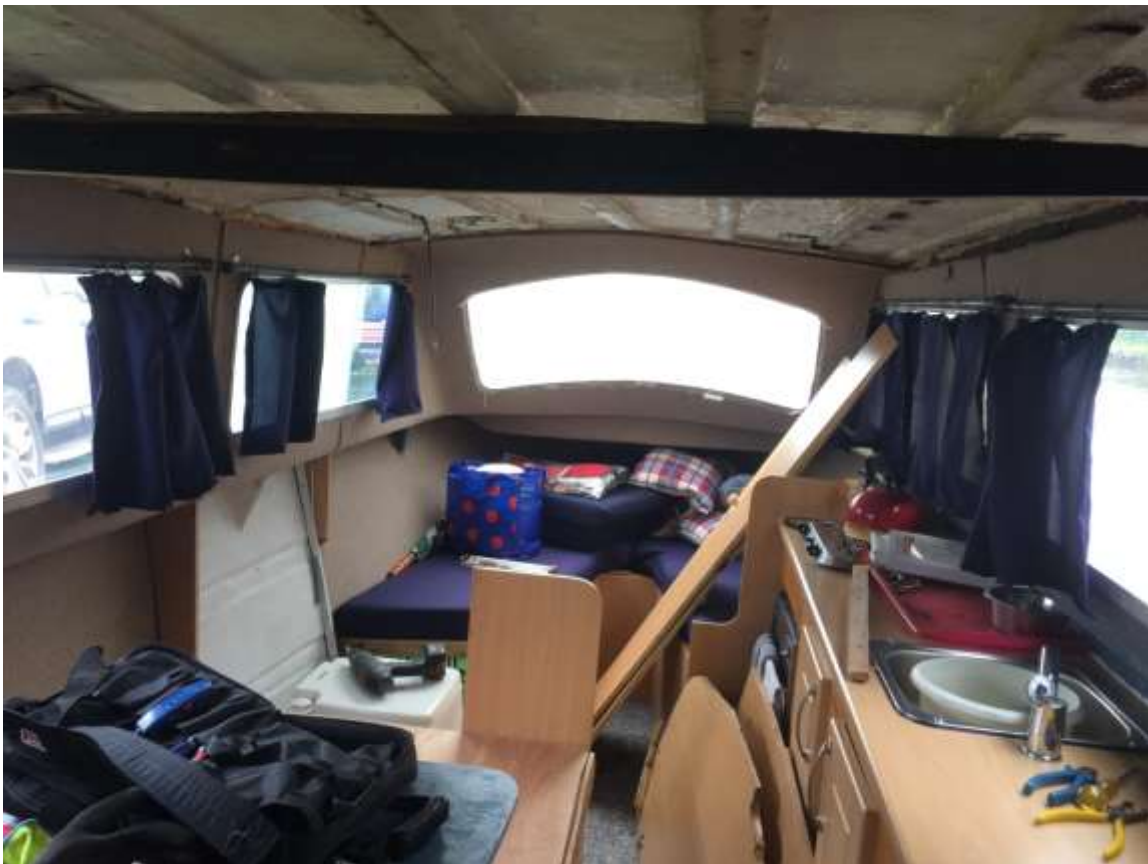
Had to strip out interior roof to gain access to Hand rail screws
