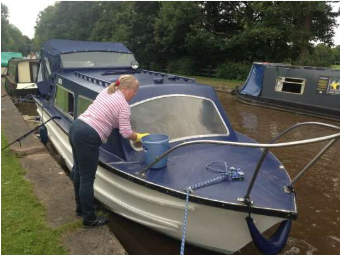
Caroline polishing the front screen. 1 st with 1000 grade wet & dry, 2 nd stage with 2500 grade wet & dry and finally with Jewellers Rouge by hand and machine Mop. 20/09/2017
