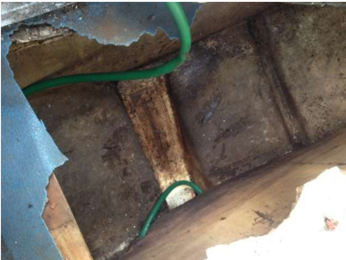
All old bilge water removed by sponging out. Bilge pipe reconnector to external fitting. All rubbish and loose material removed from below deck in cockpit and storage area. 09/10/2017
