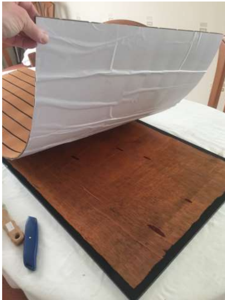
Having painted the edges black and pre-cut the EVA sheeting. These sheets have been stuck down 28/02/2018
