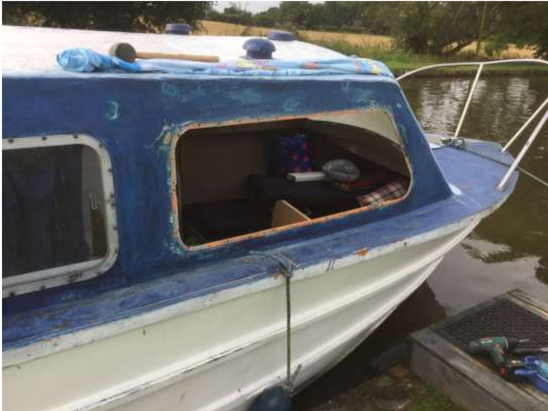
Removed all the leaking pop rivets and replaced with stainless steel nuts and bolts. Replaced old Perspex window and polished aluminium frames. (September 2019)
