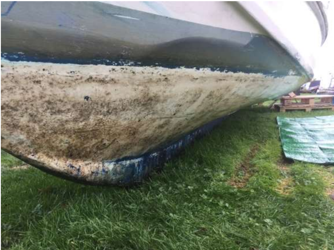
Had to scrape off all the shell fish (November 2019) Jet washed the hull prior to sanding
