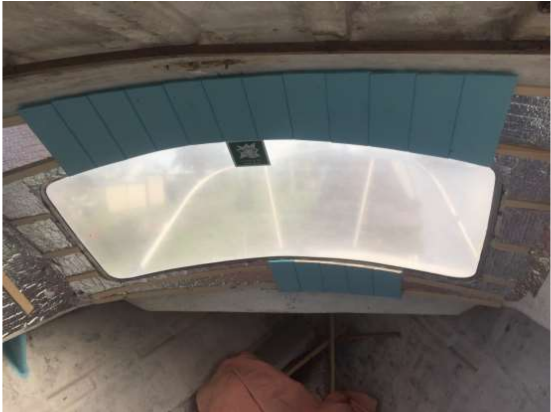
Front battened & insulated and cladding started (05/09/20) Hull side walls and knee insulated and battened (09-11/09/20)
