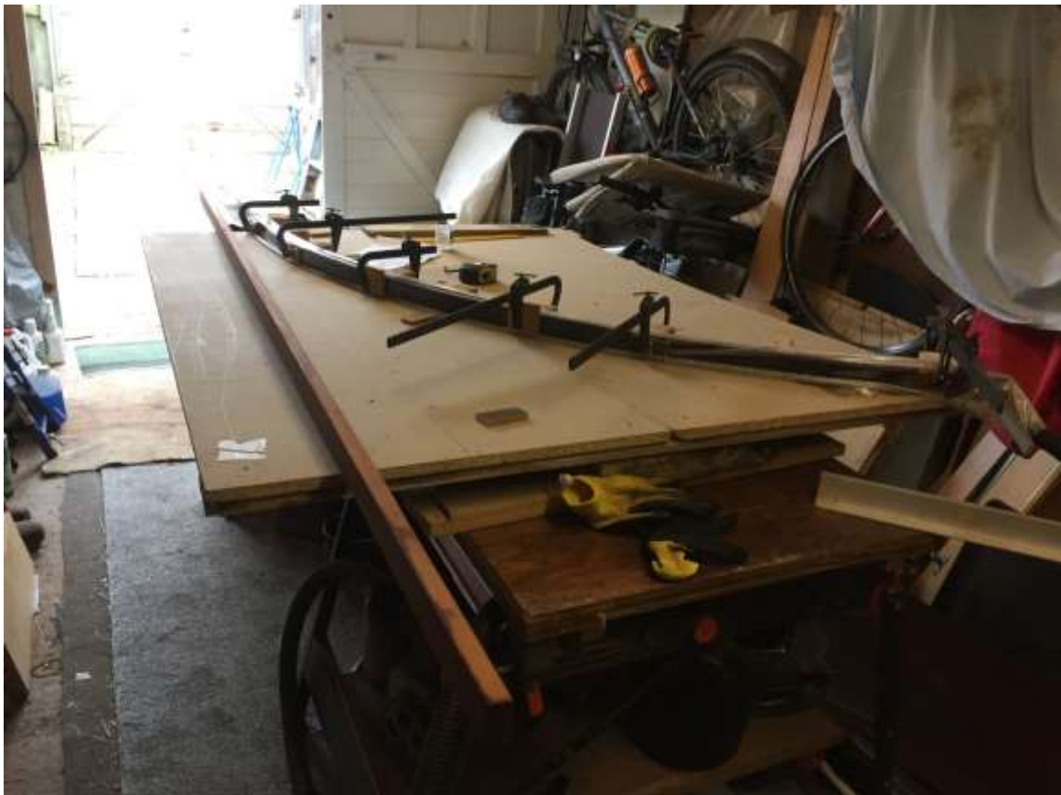
Batten whilst still in poly tube and being steamed clamped and bent to shape. Example of straight on the left and bent on the right.
