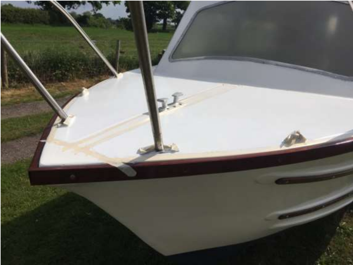
Masking up and painting anti-slip paint on decking (21/5/2020)
