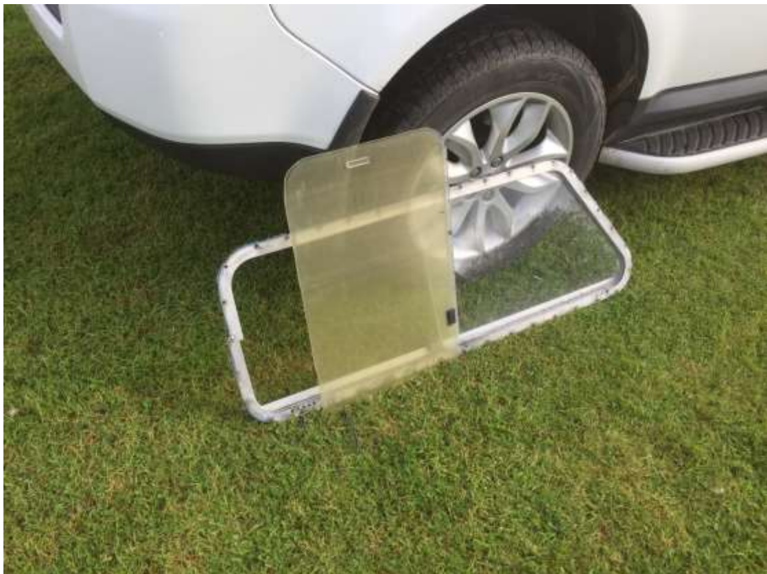
Removed all the leaking pop rivets and replaced with stainless steel nuts and bolts. Replaced old Perspex window and polished aluminium frames. (September 2019)
