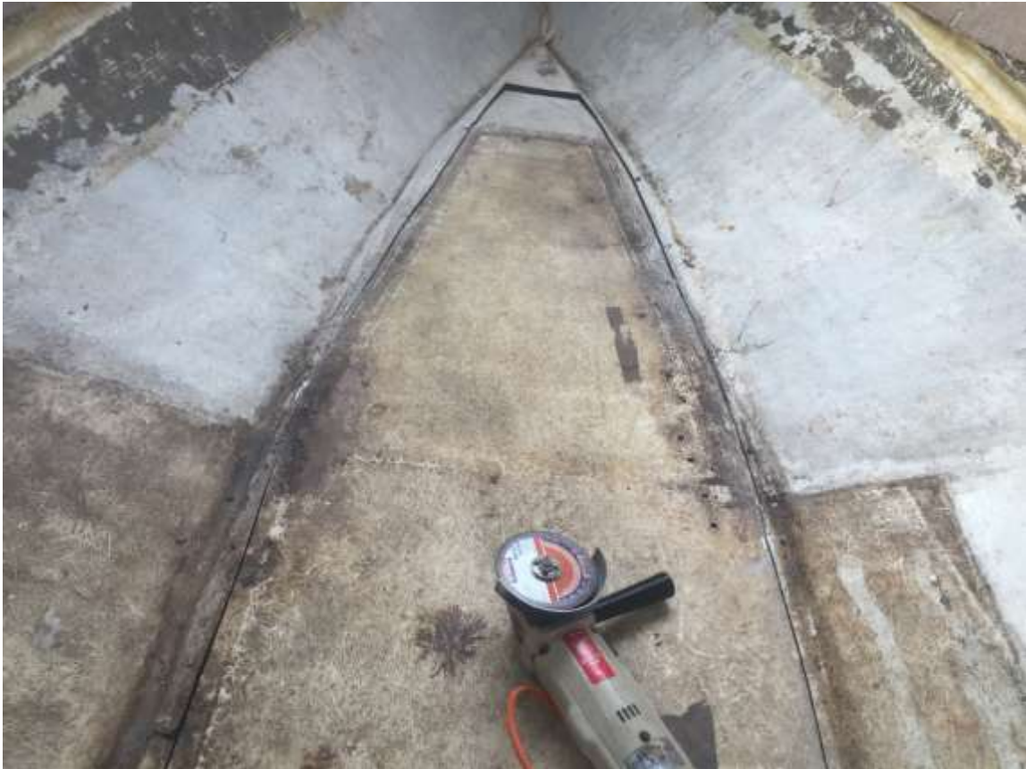
Had to cut through false floor and remove the ballast. Loose sand. (November 2019) 14 bags!
