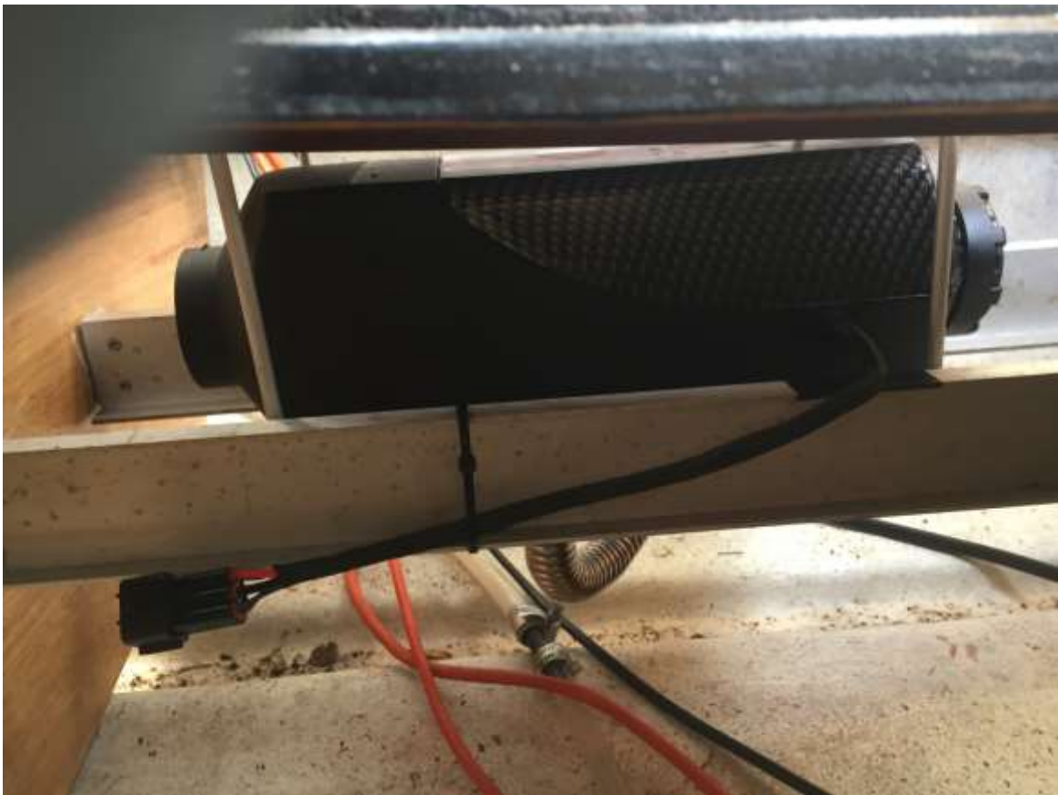
Diesel Air heater fitted below heat shield and deck.
