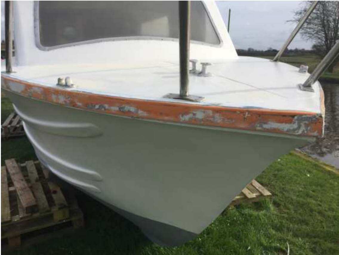
Hull primed and Gunnel stripped of sealant and loose paint (February 2020)
