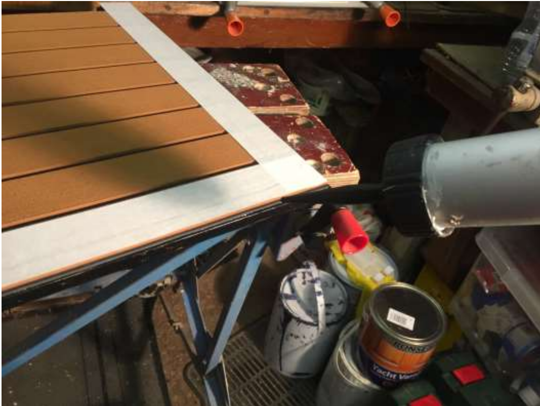
Having masked the finished surface of the EVA sheeting a bead of black sealant is applied around the edge to prevent ingress of water. 4/03/2018
