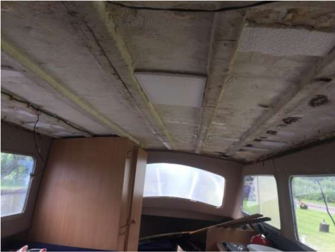
Had to strip out interior roof to gain access to Hand rail screws
