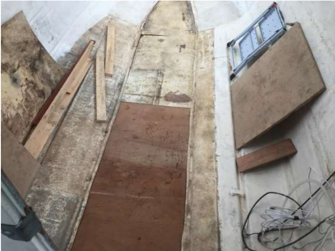
Ballast sand installed and covered with ply and then original fibre glass panels taped and glassed into place.
