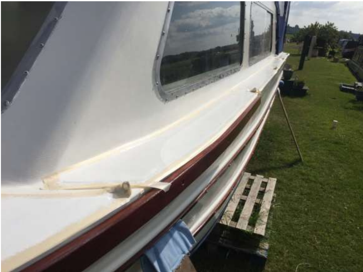
Masking up and painting anti-slip paint on decking (21/5/2020)
