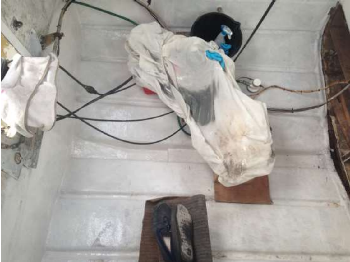
Painting the floor prior to fitting the new stringers. Removed old fibreglass tabs at the stern. 9/11/2017
