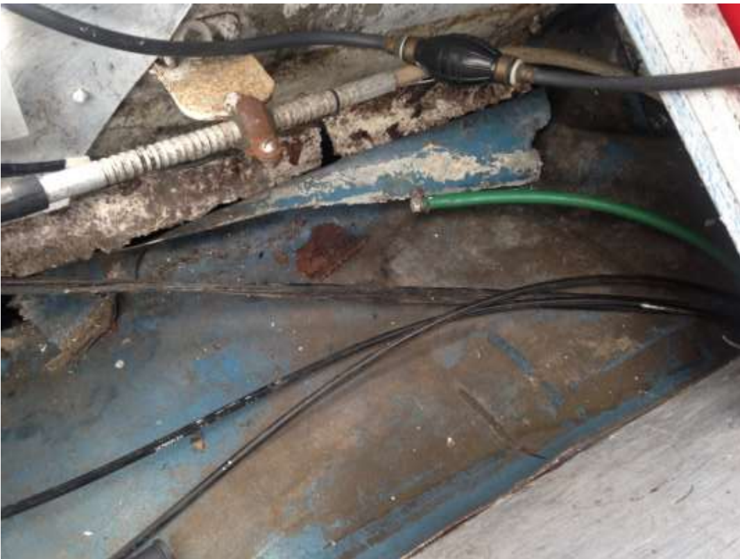
Plywood floor in storage area was hiding two previous rotten floors and their vinyl covering.
