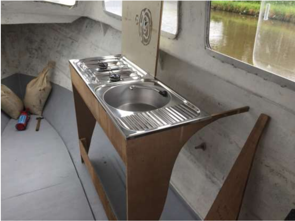
Trial fit for measurements of kitchen unit (21/7/2020) Trial fit of new kitchen unit carcass (15/8/2020)
