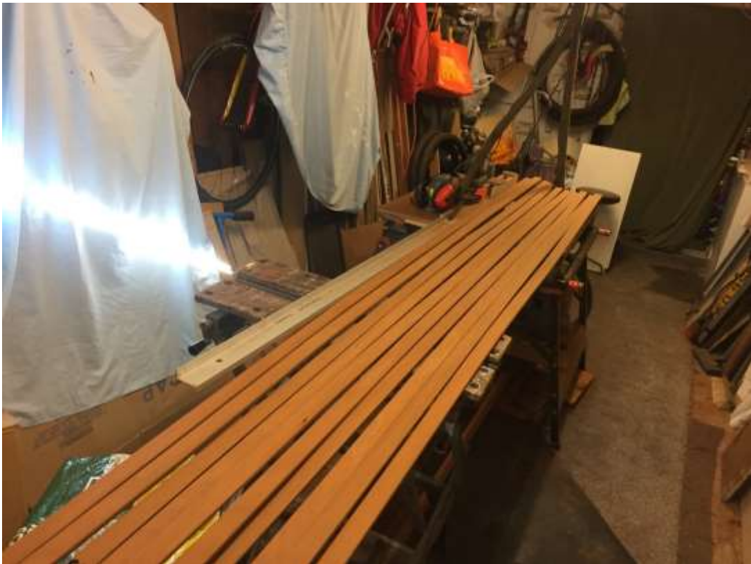
Removed deck fittings and filled holes (3/5/2020) Sanding rubbing strakes (5/5/2020)
