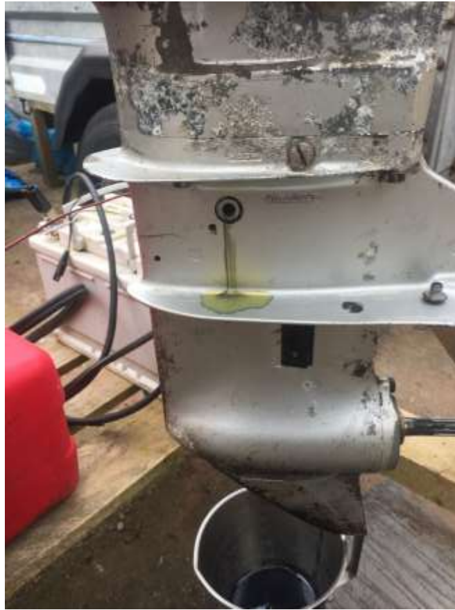
Gear box oil changed. Note the corrosion! (April 5 th 2020) Corrosion treated and primed and finished with Honda silver paint
