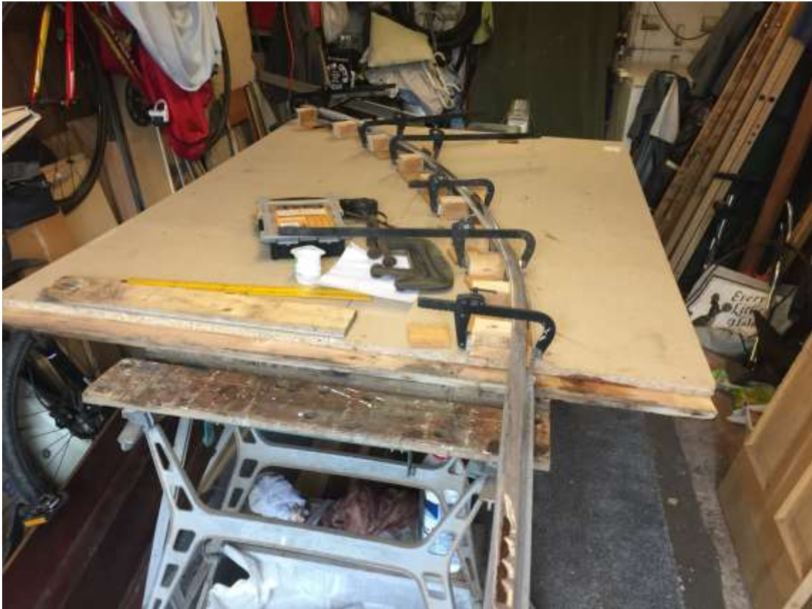
Batten whilst still in poly tube and being steamed clamped and bent to shape. Example of straight on the left and bent on the right.
