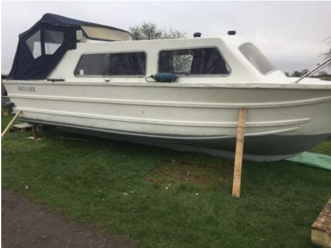
All the Gunnel rubber removed and Wooden straking removed and screw holes filled. Grey Anitfouling primer applied (January 2020)
