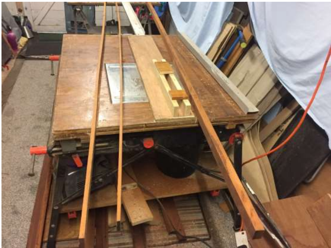
After cutting battens for rubbing strakes I made a jig to cut them into two pieces. 25/04/2020
