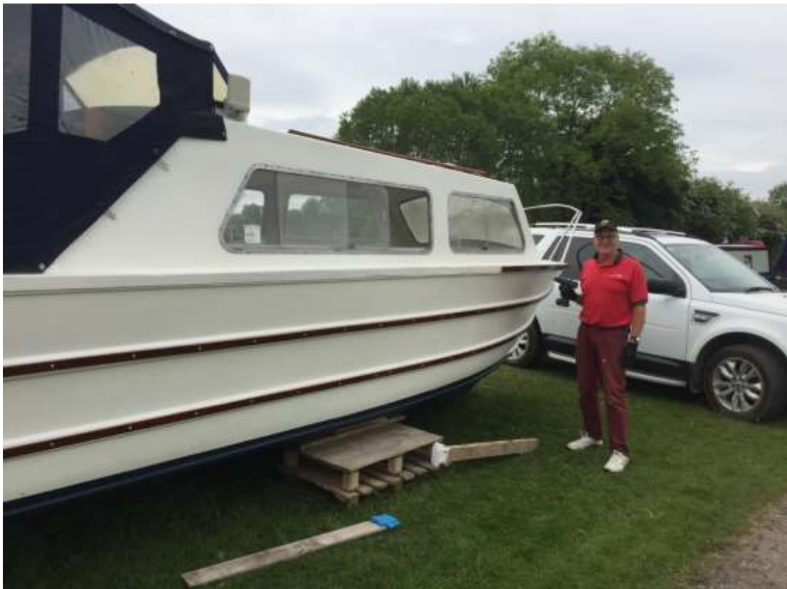
Fitted refurbished hand rails (17/5/2020) Fitting Gunwales and rubbing strakes (18/5/2020)
