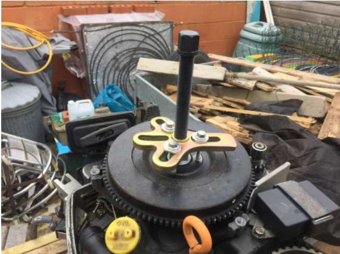
Used new flywheel puller to remove flywheel. Changed timing belt, oil, plugs, fuel filter (April 4 th 2020)
