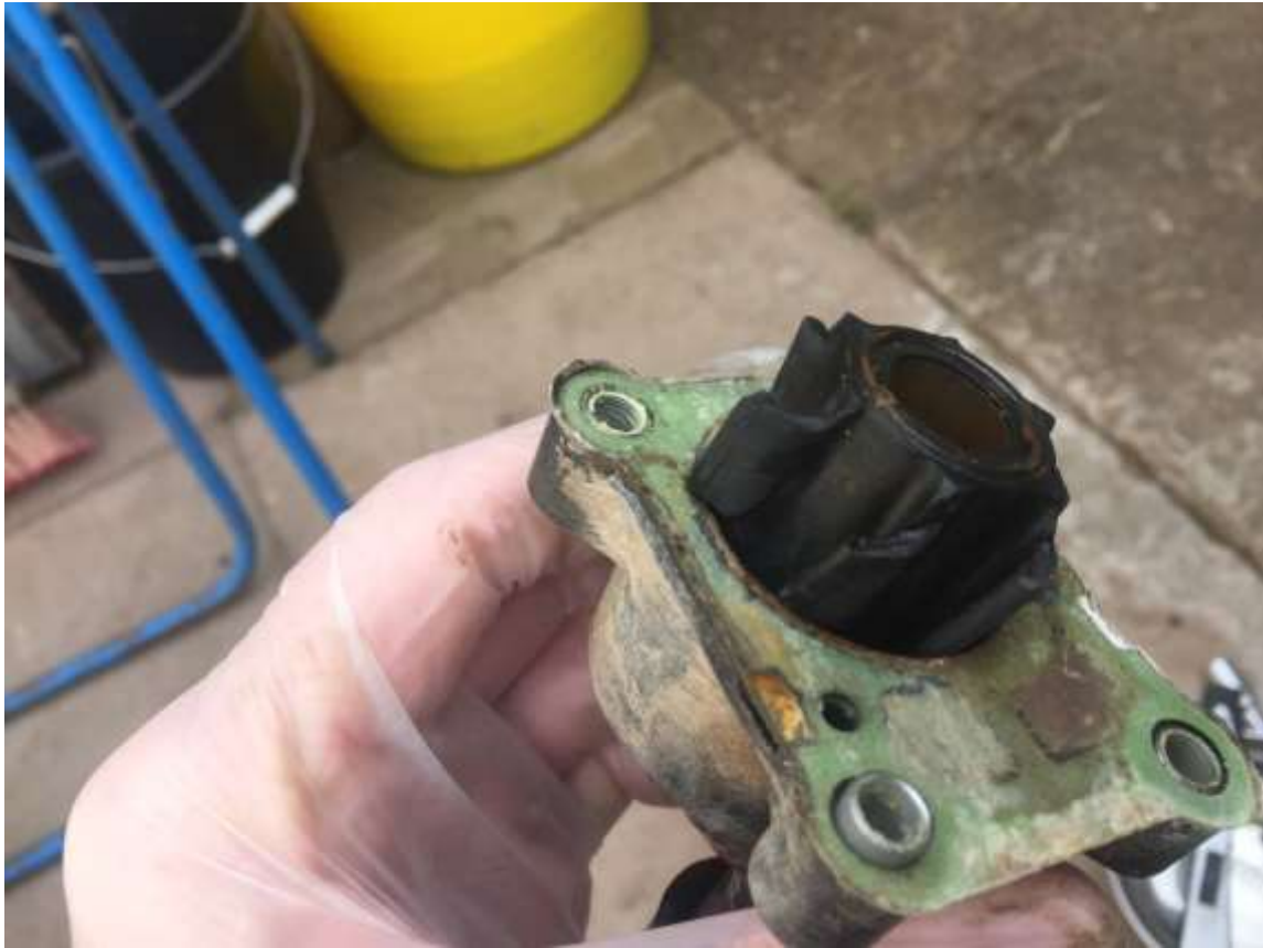
Removed bottom end to change worn out impeller
