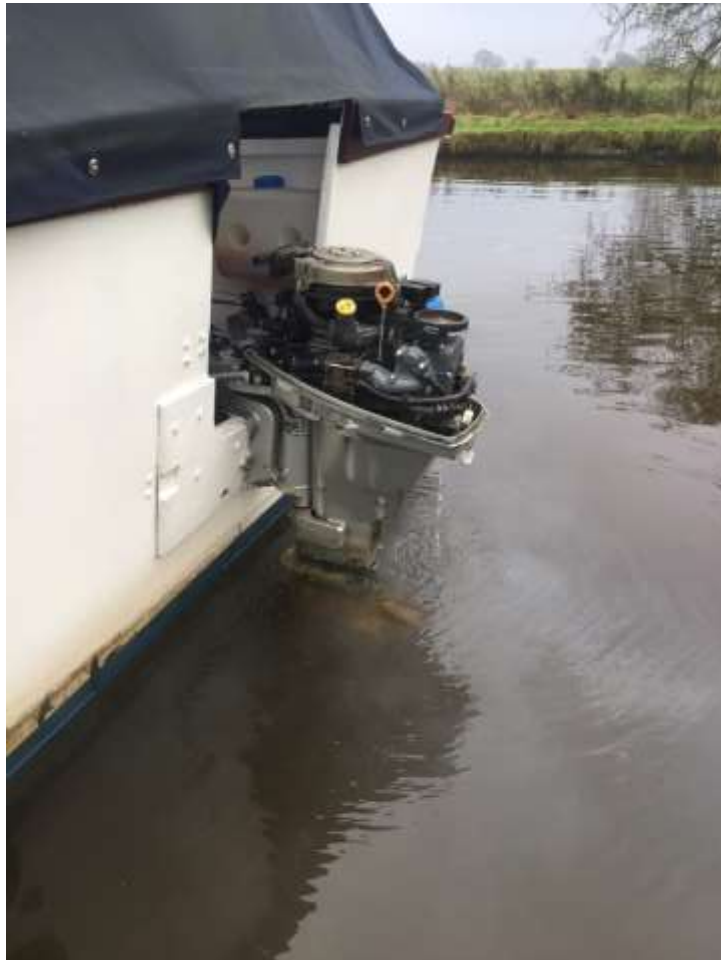
Tested outboard. No tell tale water coming out of "Pee Hole"! (5/12/20) Thermostat changed as stuck open and cleaned out manifold "Pee Hole" outlet. (7/12/20)
