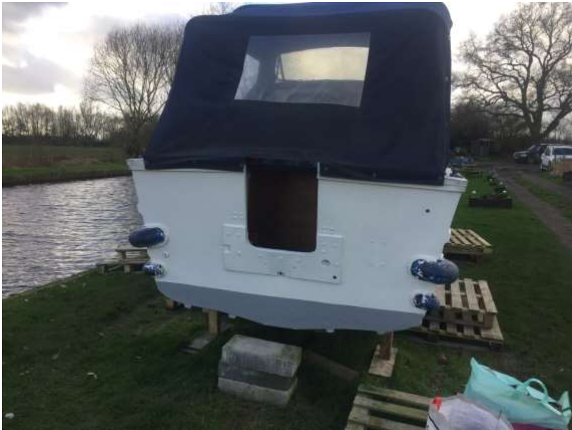
Ready for two coats of white boat paint and three coats of antifouling (February 2020)
