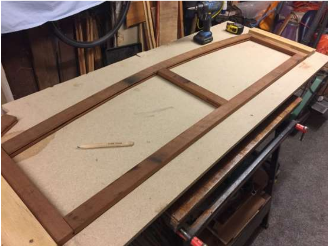
Making new windscreen frame. Steam bent top piece. (1/6/2020) Windscreen completed now designing side screens (11/6/2020)
