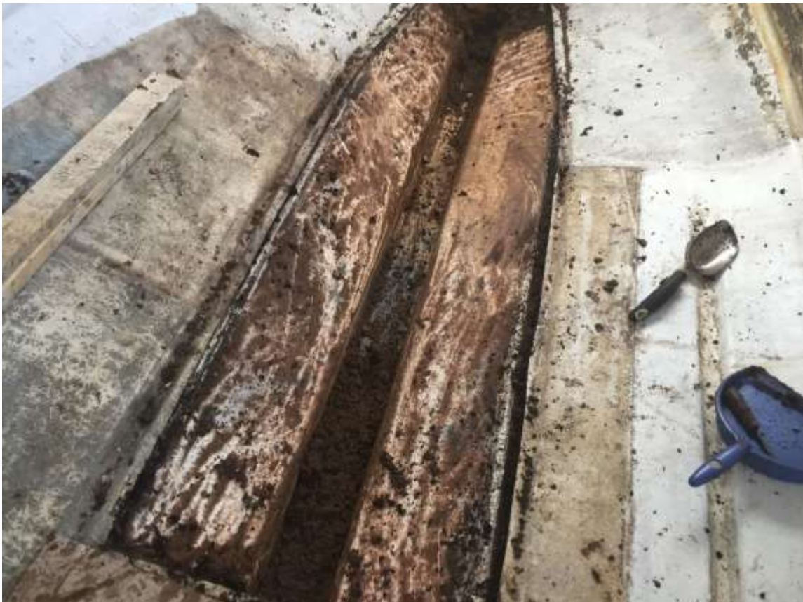
Originally there had been plywood between fibreglass and sand but this had rotted completely.
