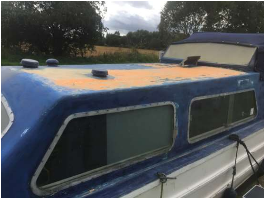
Starting the sanding down the cracked surfaces to repaint (July 2019) Had to sand roof right back to original Orange Gelcoat.
