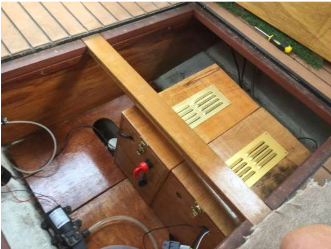
Replaced bilge floor leaving access to bilge pump. Two new battery boxes. Main and Auxiliary Batteries. (26/04/2020)
