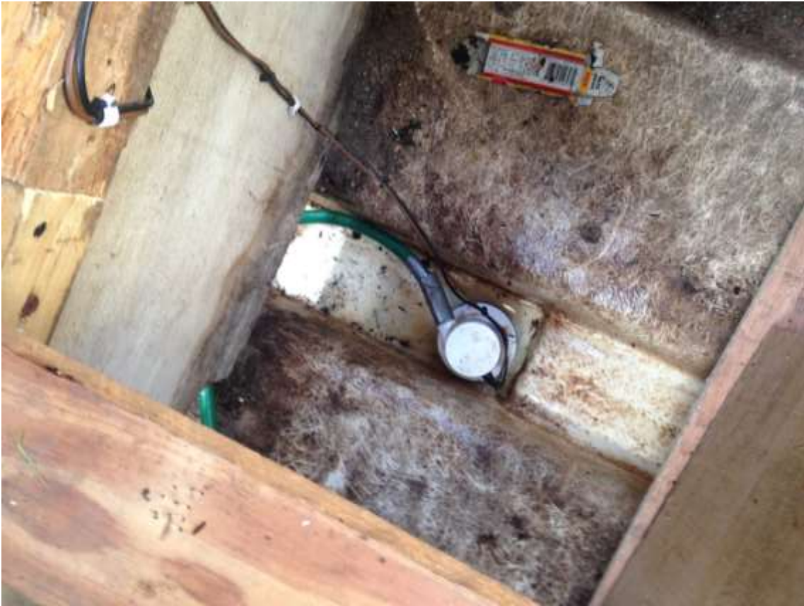
All old bilge water removed by sponging out. Bilge pipe reconnector to external fitting. All rubbish and loose material removed from below deck in cockpit and storage area. 09/10/2017
