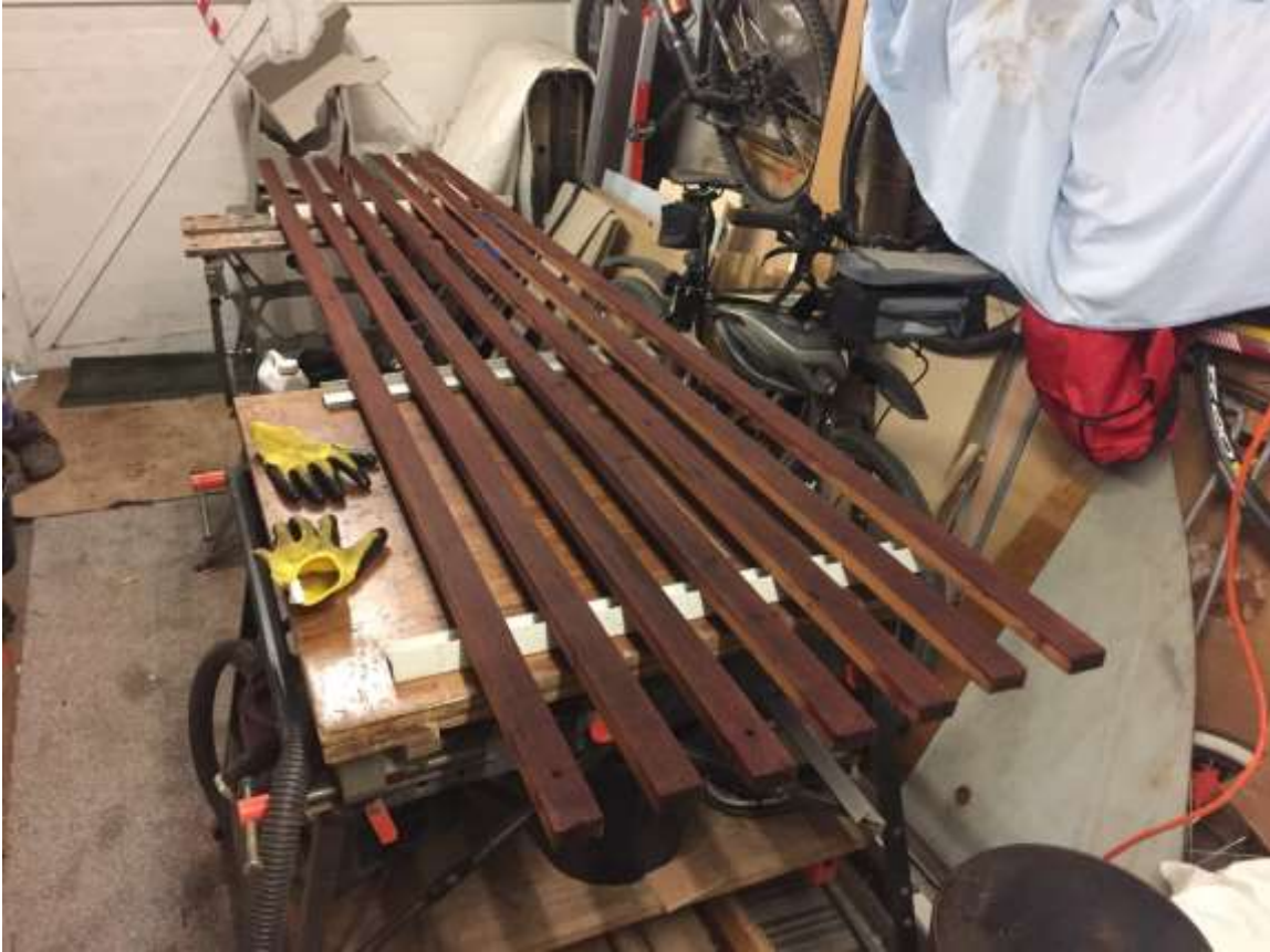
Cut battens of 7/8" x 1 3/4" Mahogany for Gunwale. Stripped old varnish and sanded. Clamping blocks glued and screwed ready for bending gunwale battens.
