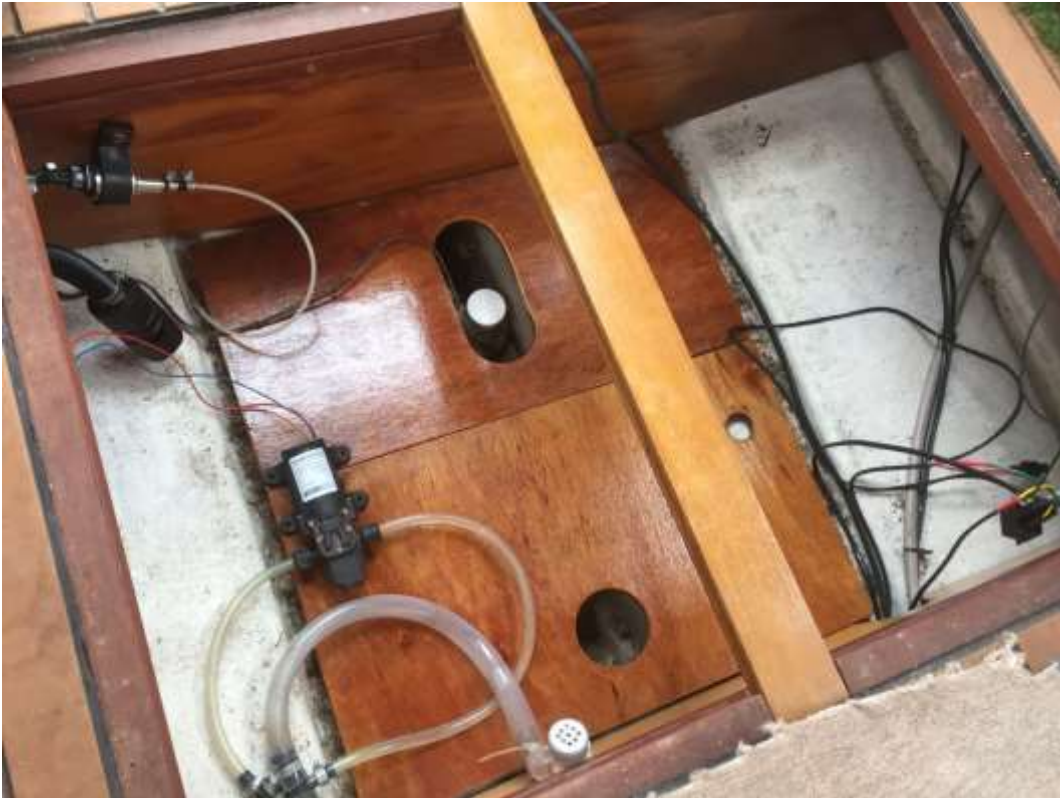
Replaced bilge floor leaving access to bilge pump. Two new battery boxes. Main and Auxiliary Batteries. (26/04/2020)
