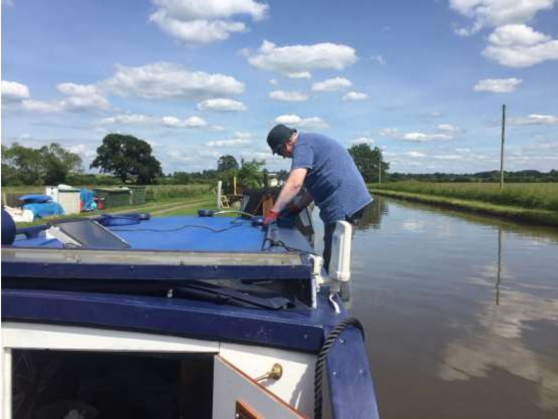
Continued sanding Striping paint off the hard wood hand rails (July 2019)
