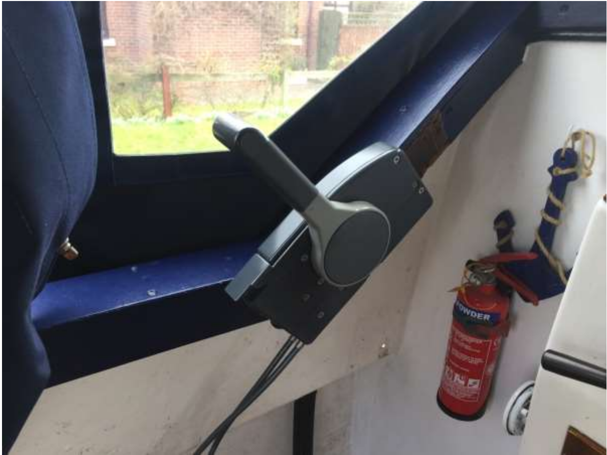
Fitted Yamaha 703 remote control. Need to convert from push to pull 6/3/2018
