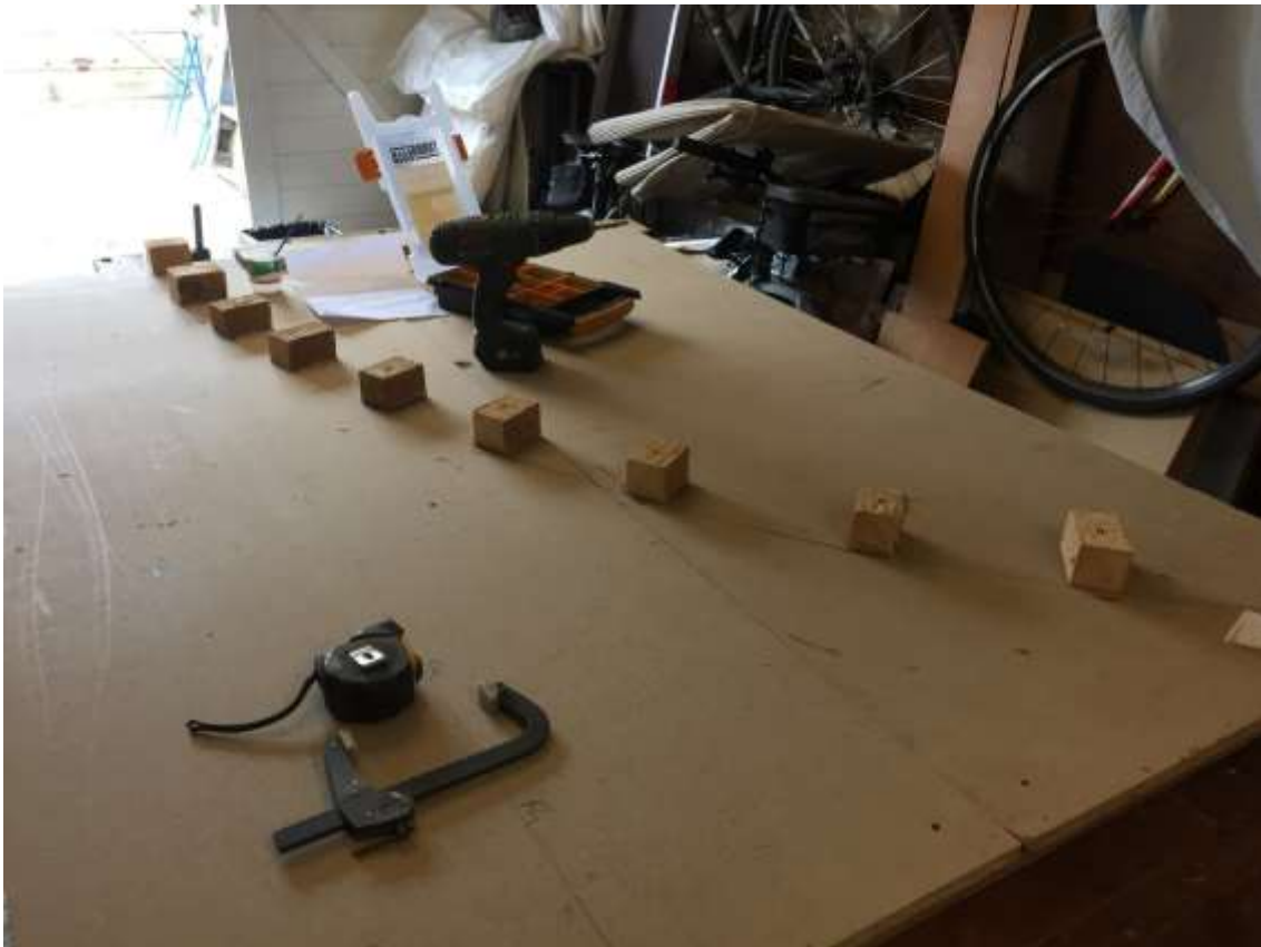
Cut battens of 7/8" x 1 3/4" Mahogany for Gunwale. Stripped old varnish and sanded. Clamping blocks glued and screwed ready for bending gunwale battens.
