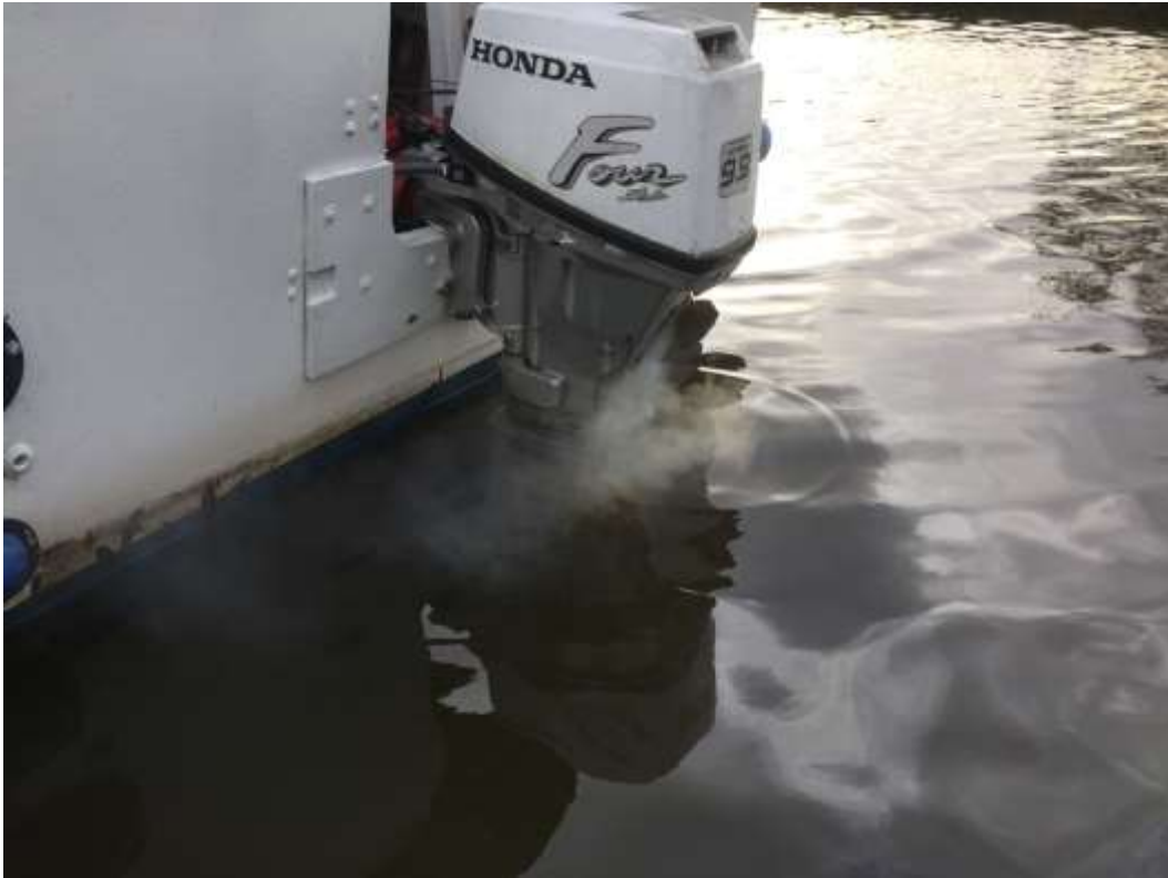
Tested outboard. No tell tale water coming out of "Pee Hole"! (5/12/20) Thermostat changed as stuck open and cleaned out manifold "Pee Hole" outlet. (7/12/20)
