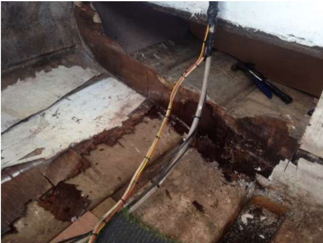
Patched up wood frames and when trying to remove to act as template all the plywood had rotted between the fiberglass. 27/10/2017
