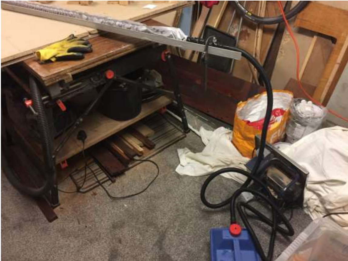
Mahogany batten placed inside layflat poly tubing and fed with steam from wallpaper stripper. Restricted steam flow out to ensure tubing inflated. Steamed for just over 1 hour.
