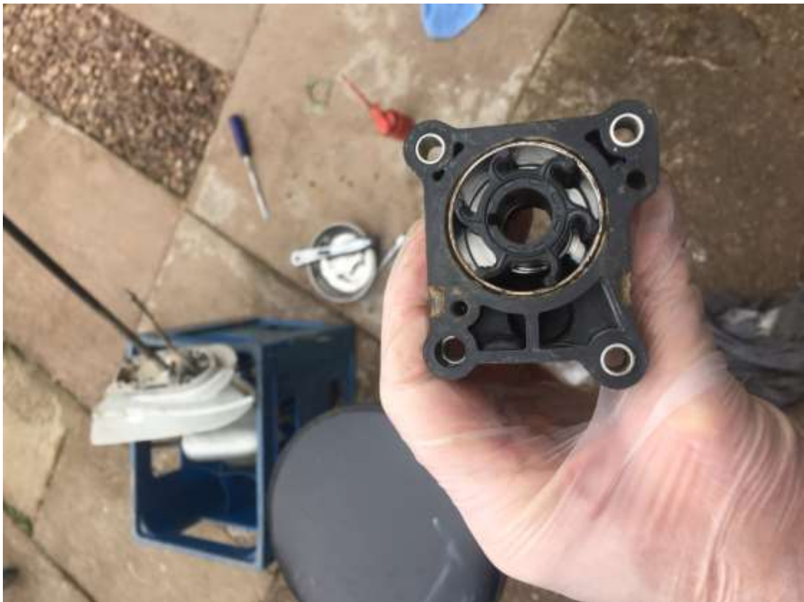
Removed bottom end to change worn out impeller
