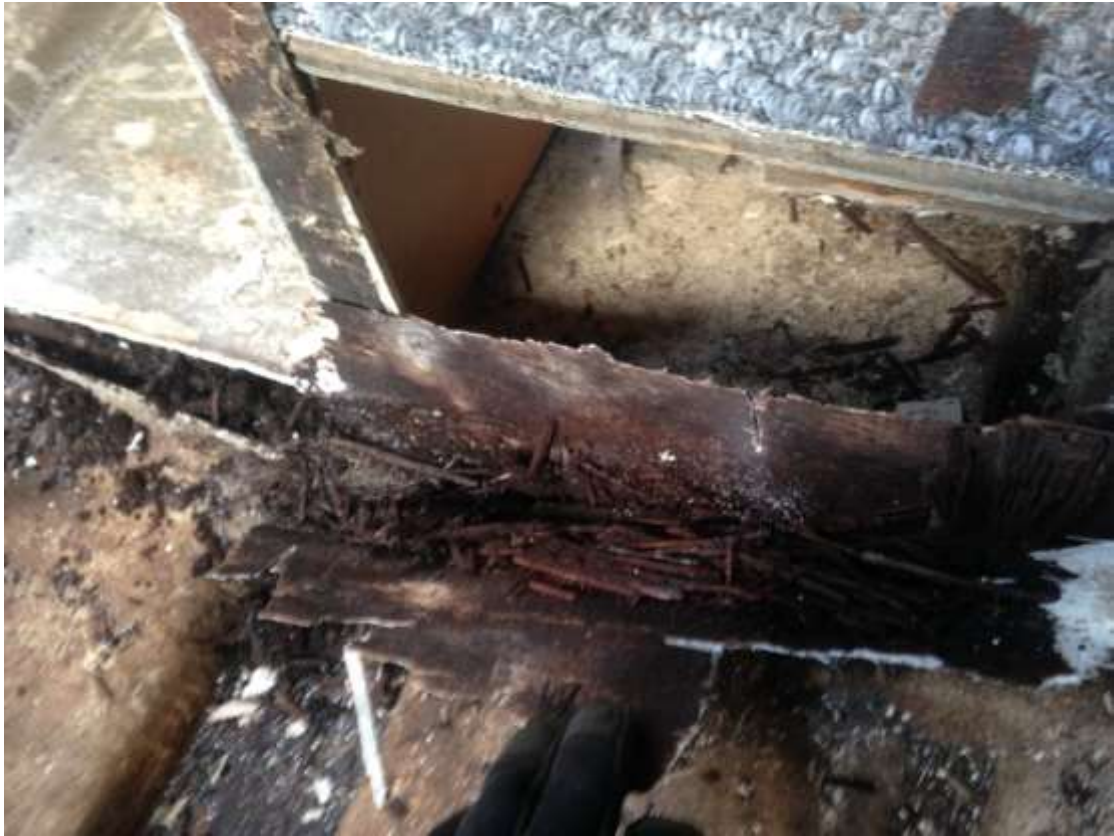
Even the rear bulkhead fell apart when removing.
