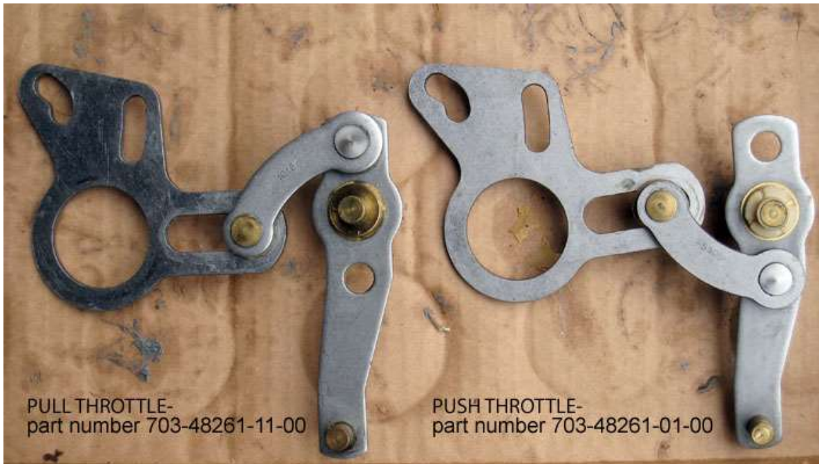
Fitted Yamaha 703 remote control. Need to convert from push to pull 6/3/2018
