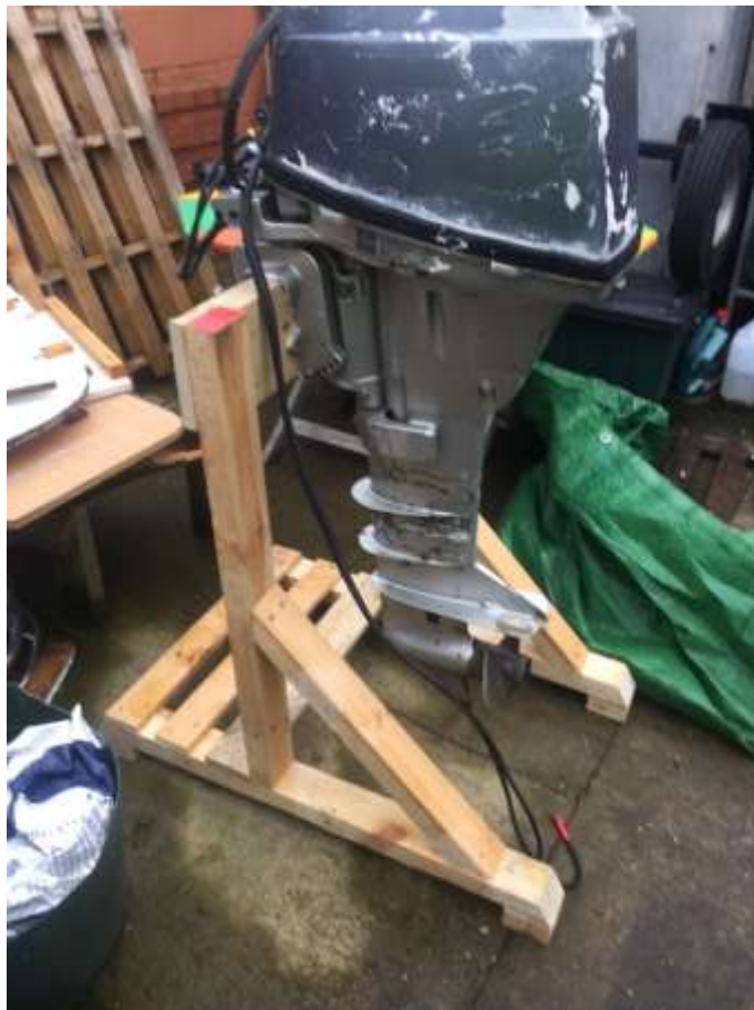
Outboard fitted to new maintenance stand ready for servicing (7 th October 2019)
