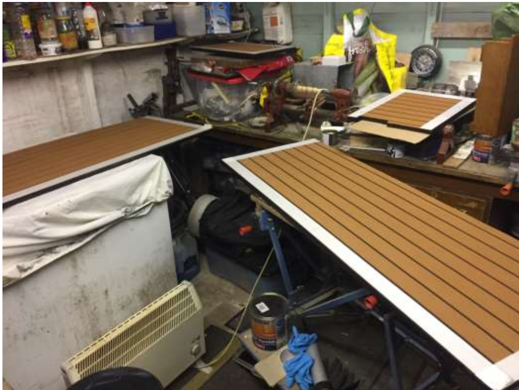
Having masked the finished surface of the EVA sheeting a bead of black sealant is applied around the edge to prevent ingress of water. 4/03/2018
