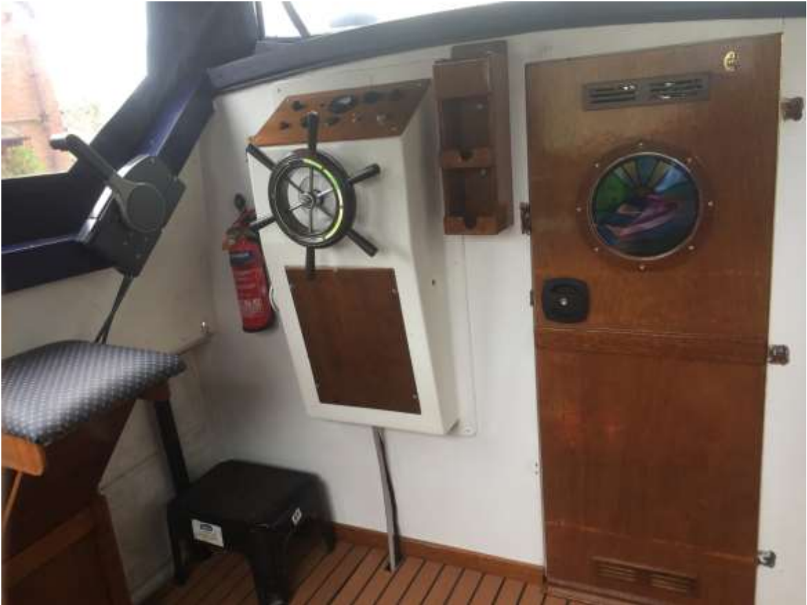
New cabin door and caravan style door lock and folding seat 23/04/2018 New seat folded away. Covered with the original rear seat vinyl. 24/04/2018
