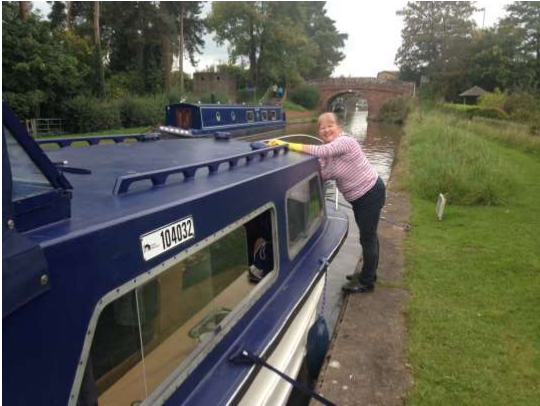
Caroline polishing the front screen. 1 st with 1000 grade wet & dry, 2 nd stage with 2500 grade wet & dry and finally with Jewellers Rouge by hand and machine Mop. 20/09/2017
