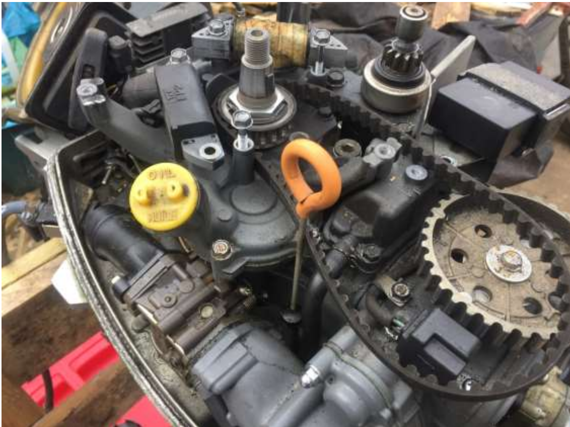
Used new flywheel puller to remove flywheel. Changed timing belt, oil, plugs, fuel filter (April 4 th 2020)
