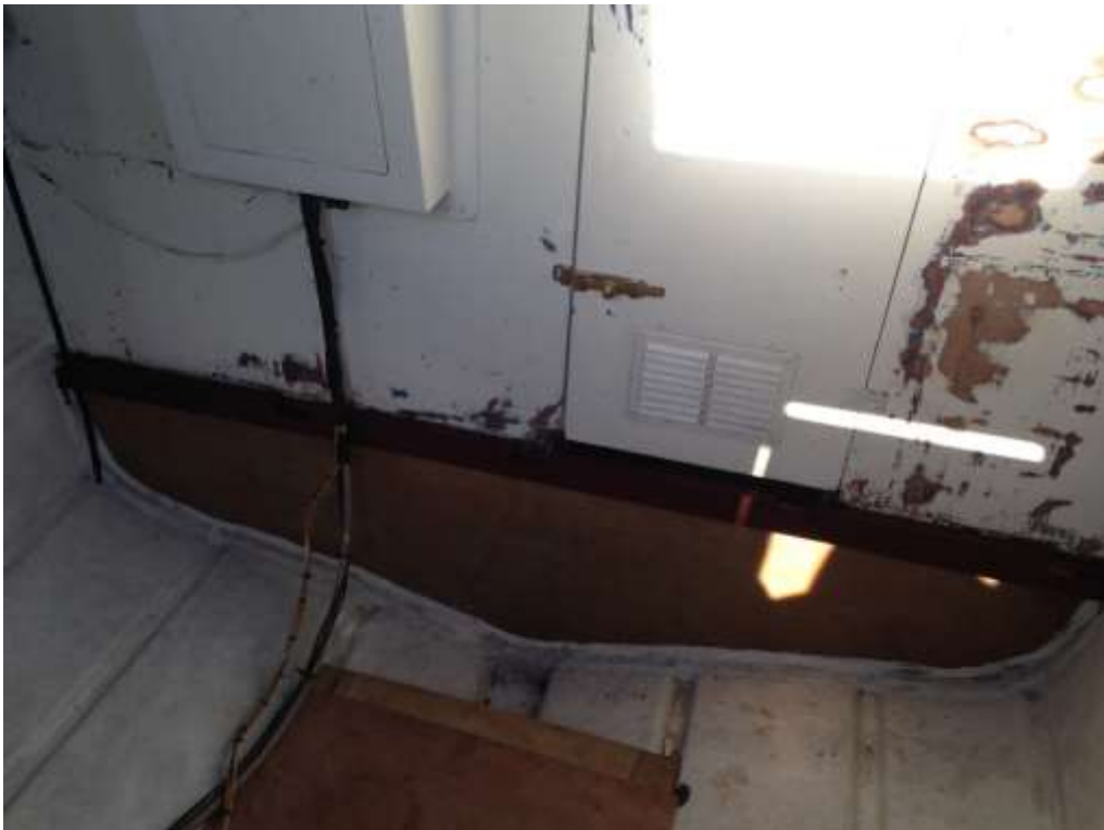
Floor stringers and supports on the canal bank. Below cabin stringer/wall fitted and bonded in forming a water tight bulkhead. 30/11/2017
