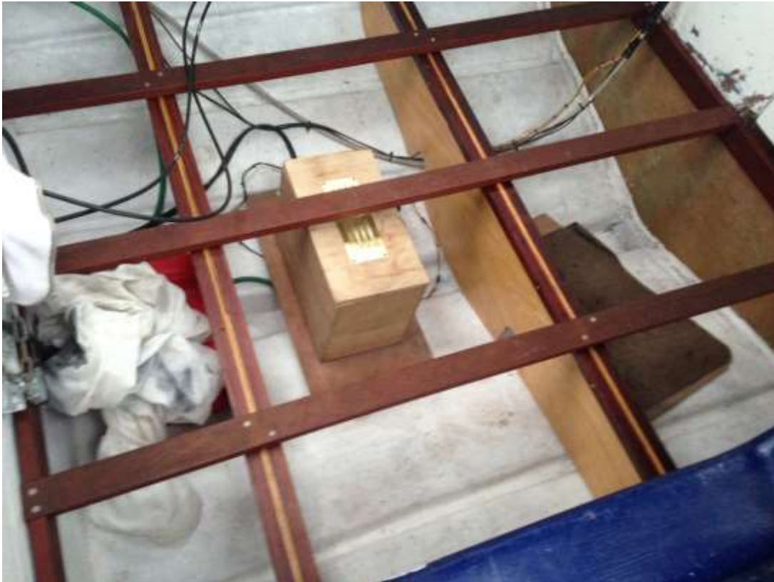
New stringers and floor supports installed in Skylark 03/12/2017. New plywood Floor installed temporarily for boat use over Xmas. 19/12/2017
