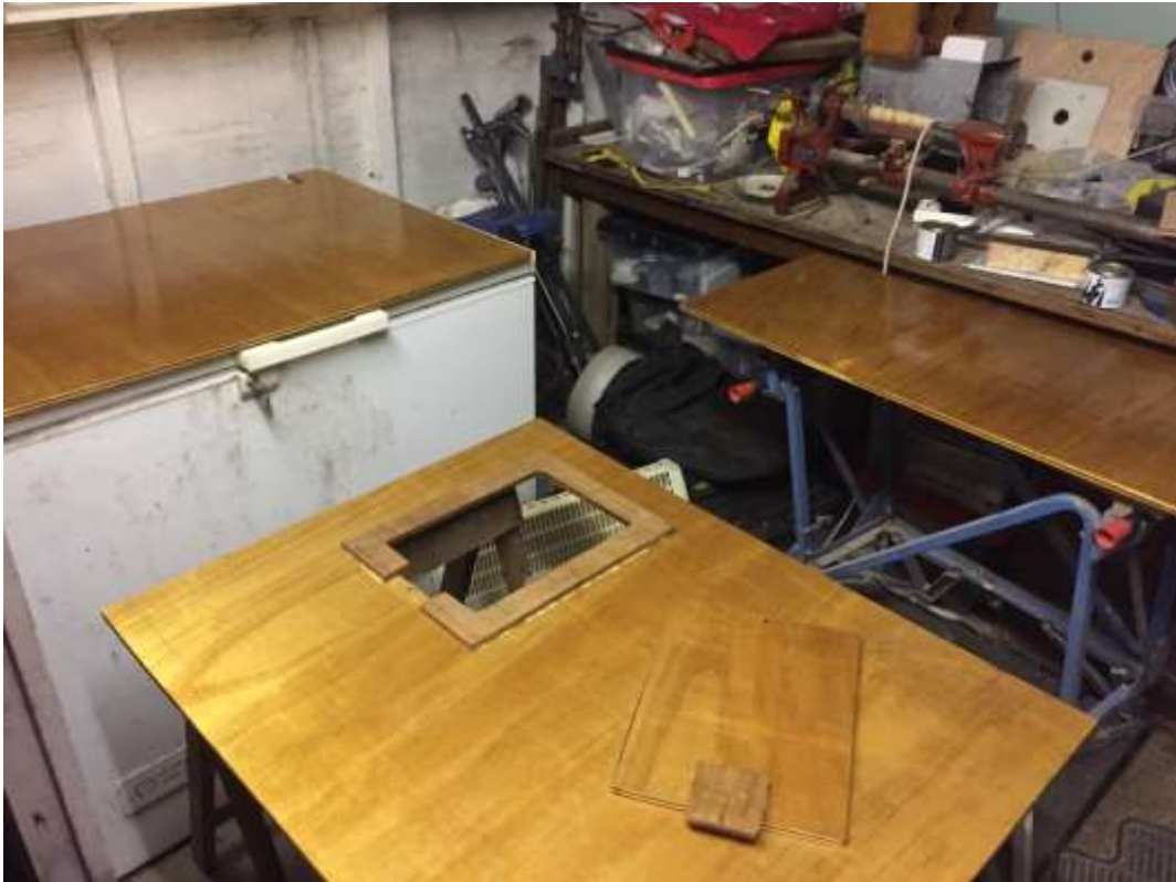
New hatch in the centre floor panel 7/3/2018 First trial fitting of Seat/step/gas locker 6/3/2018
