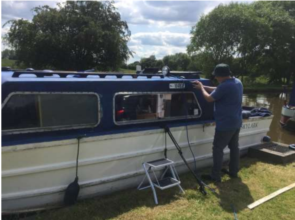
Starting the sanding down the cracked surfaces to repaint (July 2019) Had to sand roof right back to original Orange Gelcoat.
