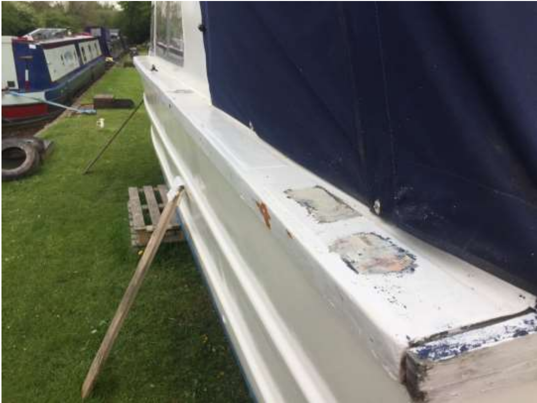
Removed deck fittings and filled holes (3/5/2020) Sanding rubbing strakes (5/5/2020)
