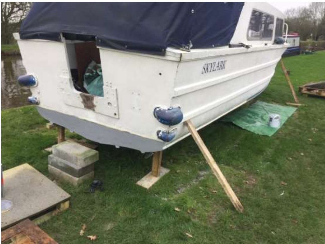
All the Gunnel rubber removed and Wooden straking removed and screw holes filled. Grey Anitfouling primer applied (January 2020)
