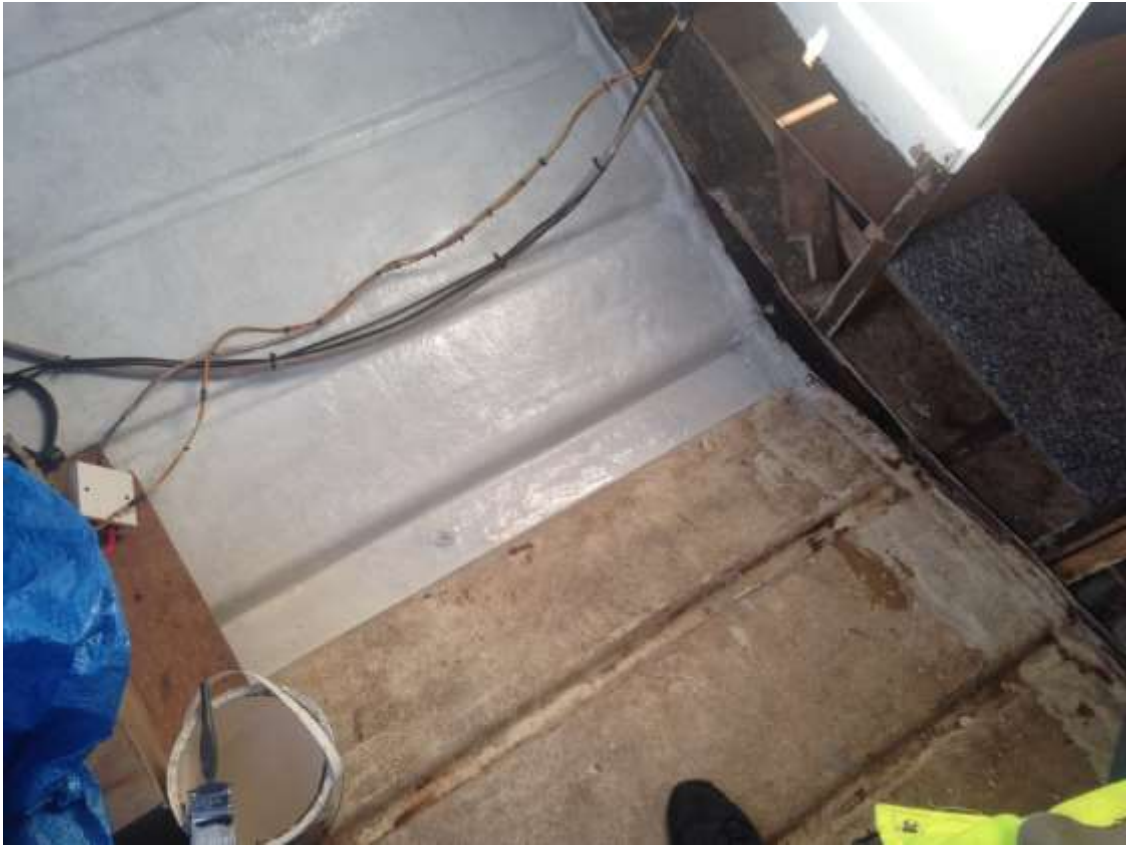
Painting the floor prior to fitting the new stringers. Removed old fibreglass tabs at the stern. 9/11/2017
