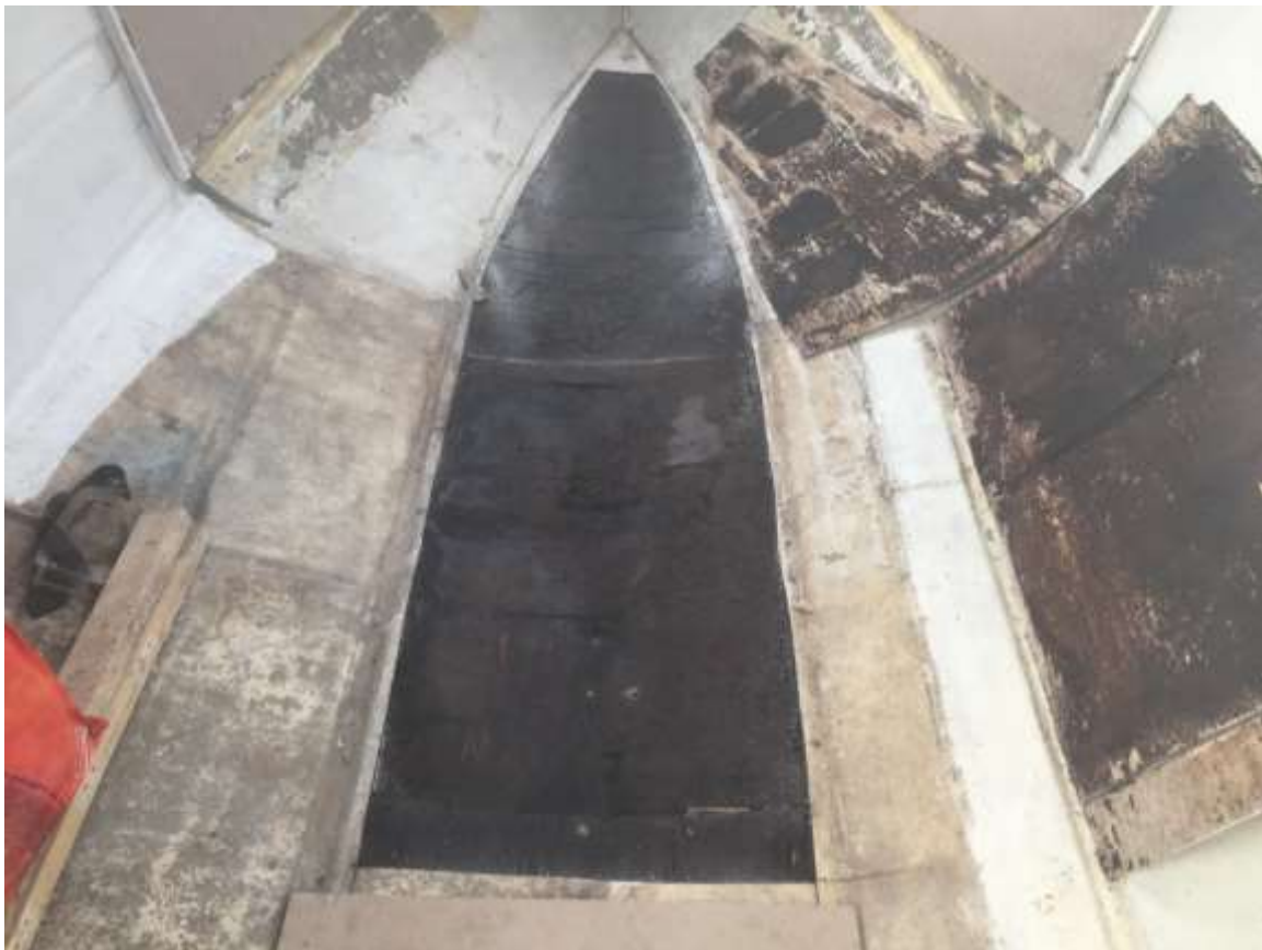
Had to cut through false floor and remove the ballast. Loose sand. (November 2019) 14 bags!
