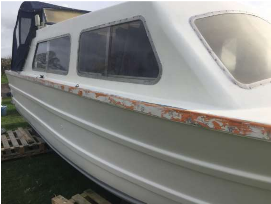
Hull primed and Gunnel stripped of sealant and loose paint (February 2020)
